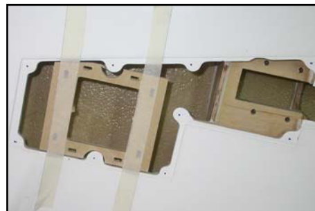
(above) Servo mount used as template for trimming servo bays. (below) Servo hatch used as template to mark fixing holes.
