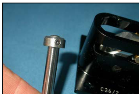
(below) Wheelcollar must be at end of pin, with bevel as shown.
