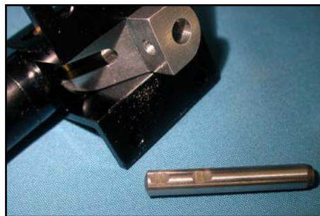
(above) You must grind small 'flats' on all the connecting pins and axles when assembling the Landing Gear. Use a drop of loctite on all set-screws for safety (below) Retract installed on the wing mount. Trim around cutout in wing as needed, and keep aligned with wheel-well.
