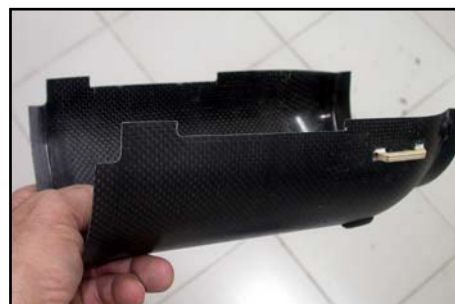
(above) Upper bypass trimmed for P80/P120 installation.
