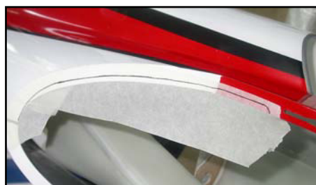
(above) The fuselage tank completed, ready for installation. (below) Trim the flanges of the cockpit area as shown to fit the the fuel tank.
