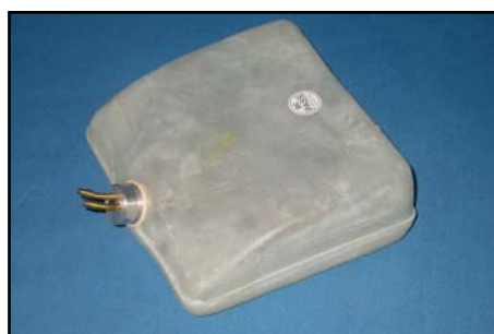
(above) Completed wing tank, ready to install in the tank bay.
