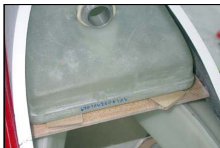
(above) Rear fuel tank support reinforced with fibreglass cloth. (below) Tack front front tank support in place with 3mm thick packers under the tank.
