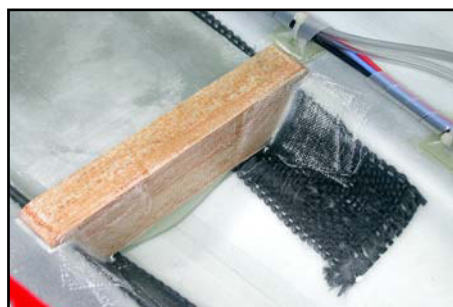
(above) Rear fuel tank support reinforced with fibreglass cloth. (below) Tack front front tank support in place with 3mm thick packers under the tank.
