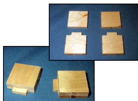
(above & below) Upper bypass ducting is secured to these 2 blocks with M3 bolts & T-nuts.
