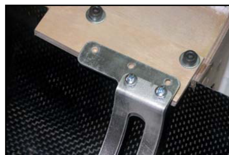
(below) Small engine mounting adapters are made by gluing the milled ply 3mm and 1.5mm rectangles together with 30 min epoxy.
