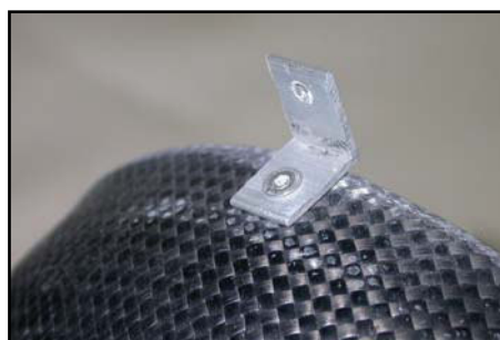
(bottom) Bellmouth brackets secured to F6 with small screws.
