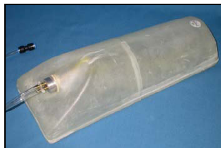
(above) The fuselage tank completed, ready for installation. (below) Trim the flanges of the cockpit area as shown to fit the the fuel tank.
