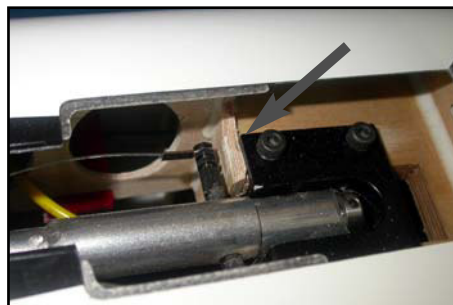
(below) Sand Bulkhead F2 for steering arm clearance if needed.
