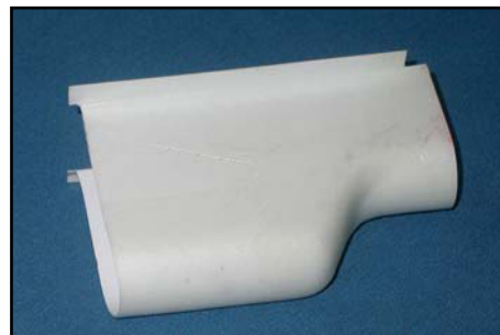
(above) Trim the moulded fibreglass leg-covers as shown to fit into the flanges in the wing.
