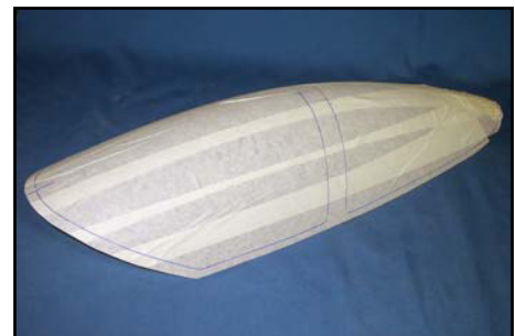
(above) Cover the clear canopy in masking tape while trimming to protect it from scratches etc. (below) Make tape 'handles' and use them to 'pull' the canopy tightly into the frame for tacking in place with odourless CA.
