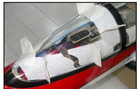
(above) Cover the clear canopy in masking tape while trimming to protect it from scratches etc. (below) Make tape 'handles' and use them to 'pull' the canopy tightly into the frame for tacking in place with odourless CA.
