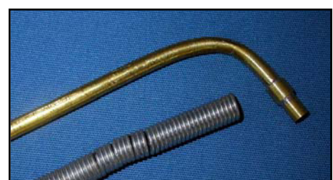
(Below) A spring is used to bend the brass tube without kinking.
