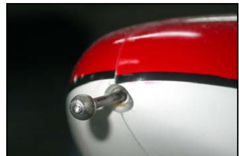
(above) Canopy frame is held to the fuselage by a 2mm wire that engages in a plastic tube - all completed at the factory for you. (below) Solder the metal ball from the ball-link onto the the wire, and countersink the hole.
