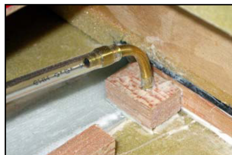
(above) Vent/overflow tube position inside the wing tank bay.
