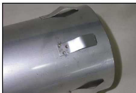
(below) Bend the 6 tabs at back of inner tube into 'V' shape.
