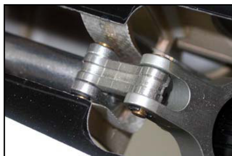
(above/below) Noseleg is centred with 'U-shape' fibreglass strip above the oleo knuckle.
