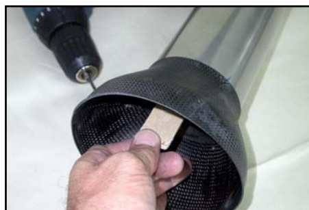
(above) Fix carbon bellmouth to inner tube with rivets or screws.
