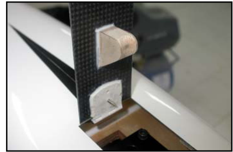
(above) Nosegear door hinge glued and screwed in position. (below) Nose door should have 1mm gap all round.
