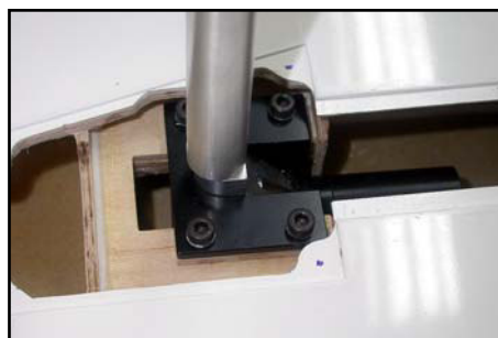
(above) You must grind small 'flats' on all the connecting pins and axles when assembling the Landing Gear. Use a drop of loctite on all set-screws for safety (below) Retract installed on the wing mount. Trim around cutout in wing as needed, and keep aligned with wheel-well.
