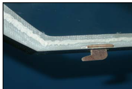
(above) Trap the inside edges of the clear canopy into the frame with a small bead of slow epoxy all around. Note also the phenolic canopy hooks seen here.
