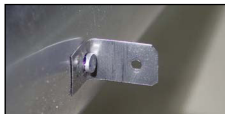
(above) Drill \varnothing 3mm hole in brackets on outer tube.
