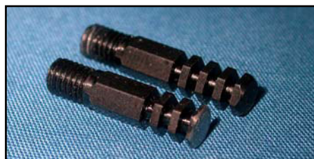
(above) Shorten steering arms. (below) Grind flats on connector pin for steering arms as shown. (bottom) Nosewheel oleo with axle and centering tubes.
