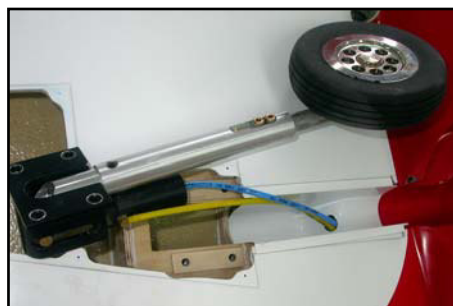
(below) Fibreglass leg covers trimmed and trial installed in wing for final adjustment. You can also see the ply packers used to adjust height of wheels in wheel-wells.
