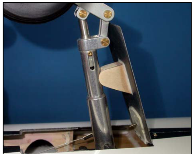
(above) Block is made from sandwich of 0.8mm plywood and 10mm balsa. Shape as shown. (below) Adjust thickness of block and depth of radius so that door just clears oleo knuckle when opening, and closes completely.
