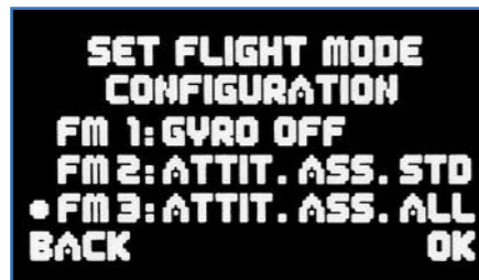
The default Flightmode configurations of the iGyro for different plane types. In the above picture, the standard set-up, below Vector Thrust.
