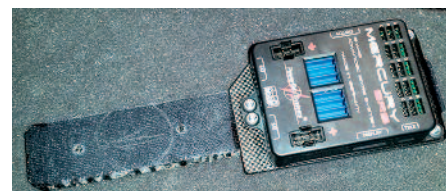
The Mercury is located in a CFRP sandwich carrier, behind the Canard frame of a J-10. The cardboard holder can be used as a stencil.
