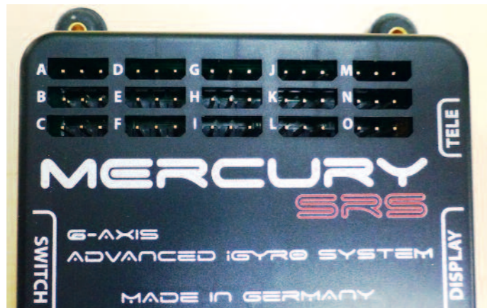
15 assigned servo outputs of the Mercury SRS.
