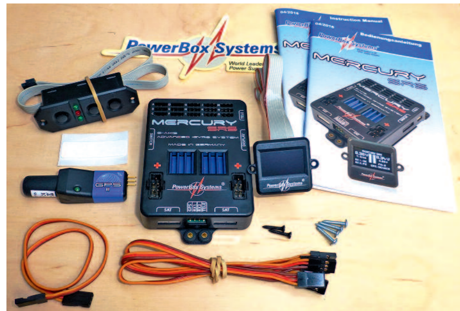
The delivery scope of the Mercury SRS from PowerBox Systems with GPS II sensor.
