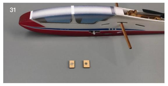
32. Install the fuselage magnet seat.
