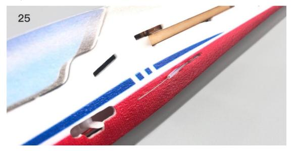
26. Install the pushrod clip on the rudder control horn and connect it with the wire by using a heat shrinkable tube.
