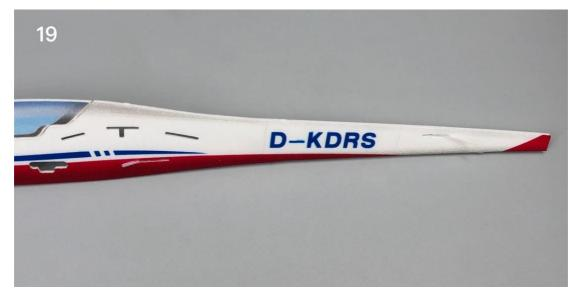
20. Close the fuselage on both sides and glue. Pay attention to keep the fuselage edge aligned with the fuselage side panel edge. Check to eliminate the distortion of the vertical tail.
