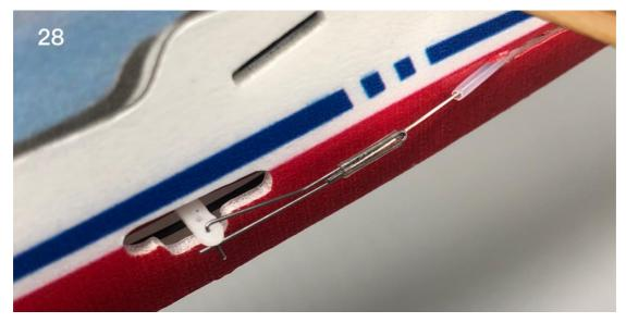
29. Cut off the connection points on the side of the hatch cover so that it can be lifted forward.
