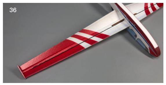
36. Attach a 250mm carbon fiber rod on each bottom side of wings.
