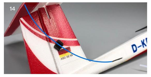
15. Glue the conduit to the conduit base inside the fuselage, and the two ends of the conduit pass through the two conduit holes on the right side of the fuselage.Left end of the guide pipe extends out of the fuselage by 5mm.
