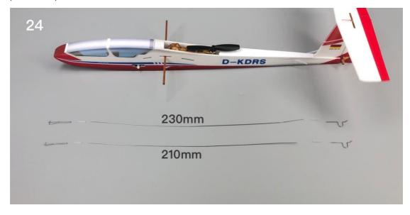
25. Thread the steel wire into the conduit on the fuselage. The steel wire is used for elevator drive, and the shorter one is used for rudder drive.
