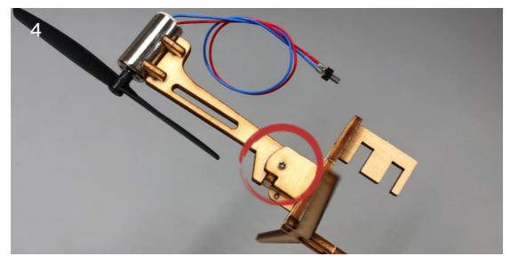
5. Screw in another m1.2x6 screw from the right side to form the motor line limit to prevent the motor line from interfering with the motor base movement or propeller running.
