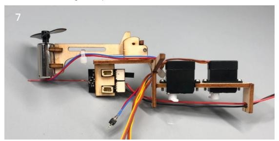
8.Connect the cable of servos and motor, and connect the receiver to power for test. Ensure that the servos and motor work normally and the motor rotation direction is correct. Secure the cable with ties.
