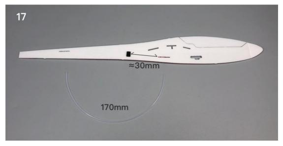
18. Glue the conduit to the conduit base on the left side of the fuselage, both of the ends of the conduit pass through the conduit hole.
