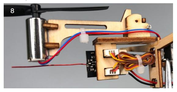
9. Combine the fuselage inner structure with the right panel of the fuselage.
