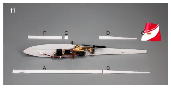
12. The installation of fuselage side plate is completed, as shown in the figure. Take 200 mm conduit and two duct seats for elevator drive.
