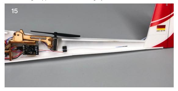
16. Glue the end of the duct to the duct seat on the vertical tail.
