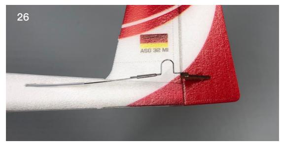
27. Connect elevator control horn, pushrod clip and steel wire.
