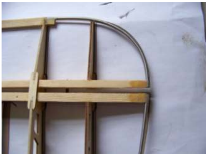
(10) Bend the 4mm stainless steel tube according to the installation drawing, then glue to the wing. Suggest using fiber cloth to strengthen the sticking-joint.
