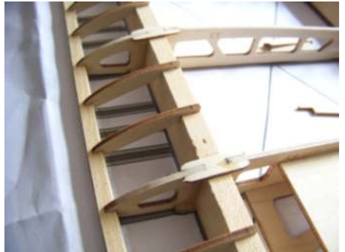
(9) Joint and glue the half ribs.
