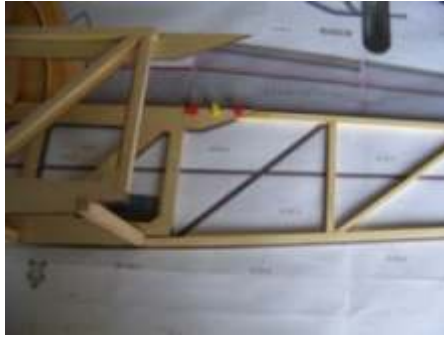
(9) Joint the retral frame of fuselage with battens according to the installation drawing. Then connect it on the fuselage.
