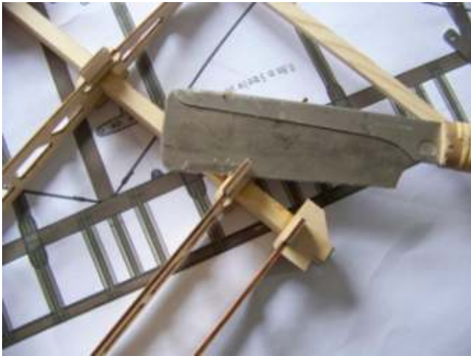
(3) Cut the redundant wood until the wing assembly is finished and the glue dries.
