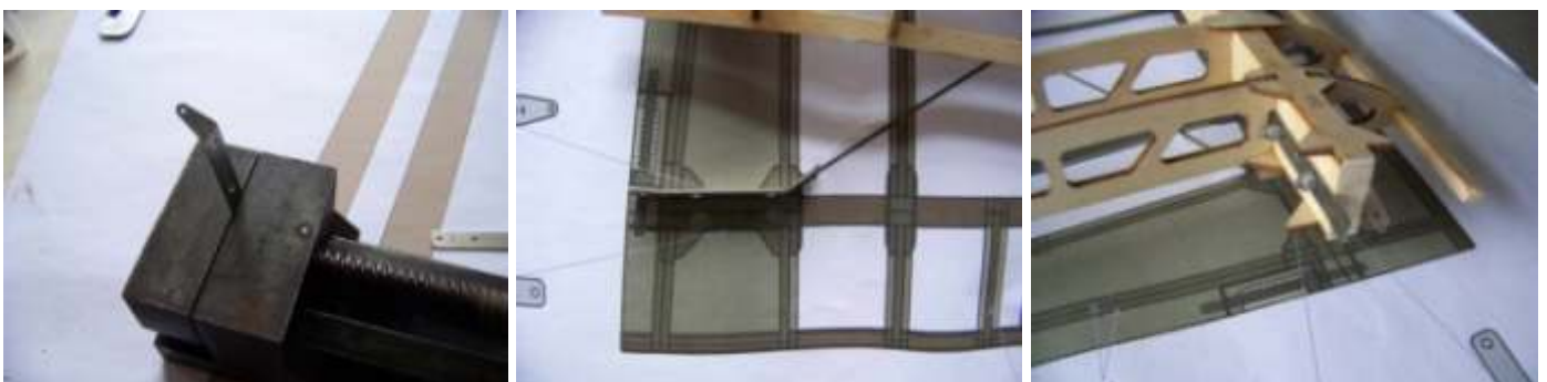
(7) Make the metal parts and fix them with screws.
