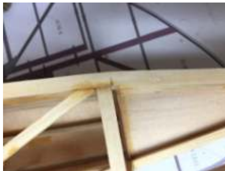
(13) Make a small cut for bending the battens easily. Then joint A23*2 & A24 , and the diagonal pillars, strengthening plates like the pictures.
