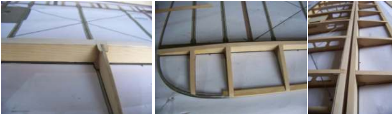
(15) Glue balsawood sheet on the aileron girder and smooth it. And then glue 1mm plywood sheet on it. (Same steps as the wing girder.)
