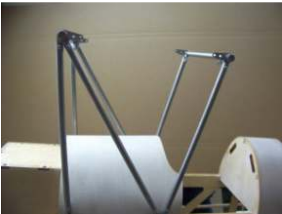
Supporting for the fuel tank.
