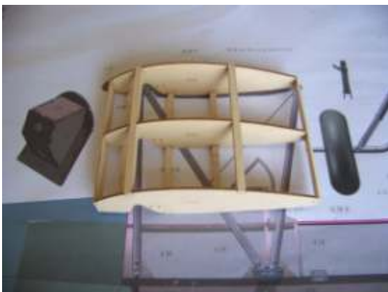
(6) Joint and glue the parts like the picture and then glue the 1mm plywood sheets cover.
