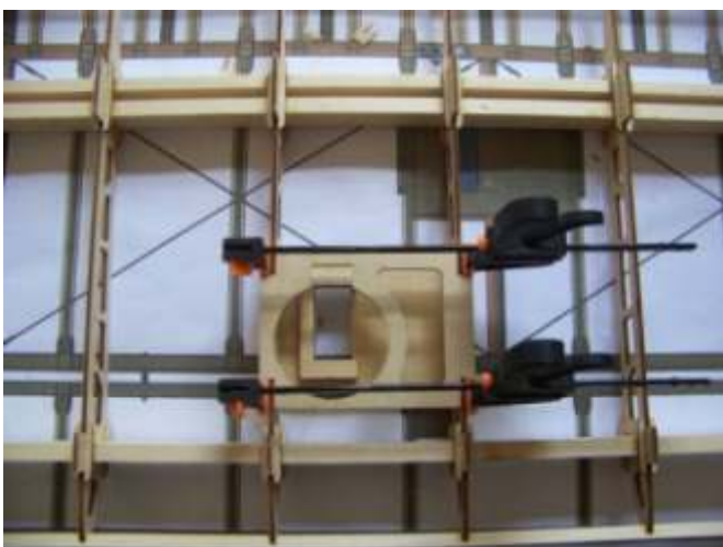
(8) Overturn the wing and install the servo mount cover.
