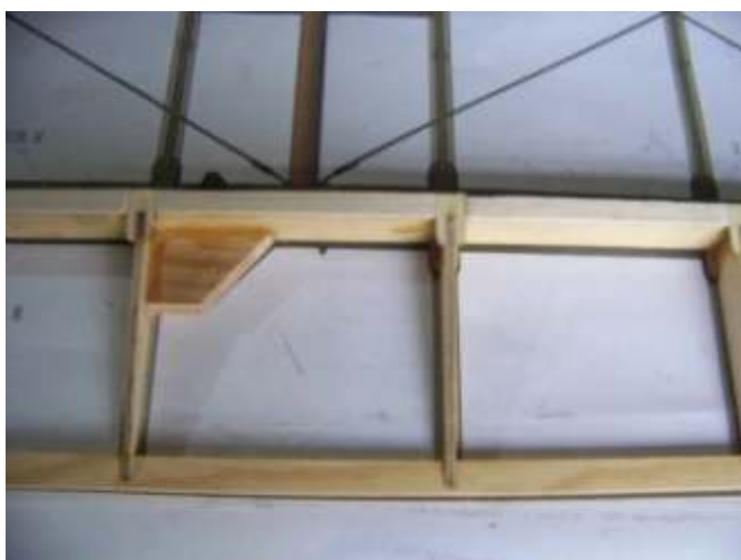
(14) Joint the strengthening plate for servo horn.
