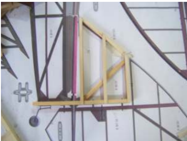
(7) Sand the vertical fin front batten to be cambered.
