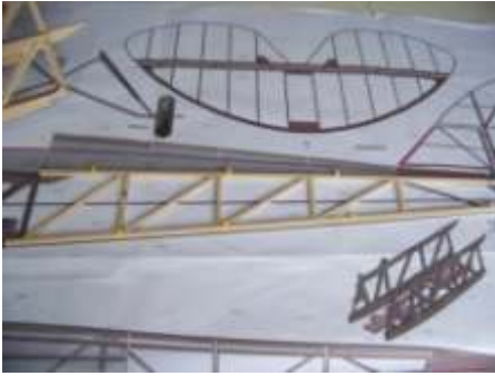
(9) Joint the retral frame of fuselage with battens according to the installation drawing. Then connect it on the fuselage.
