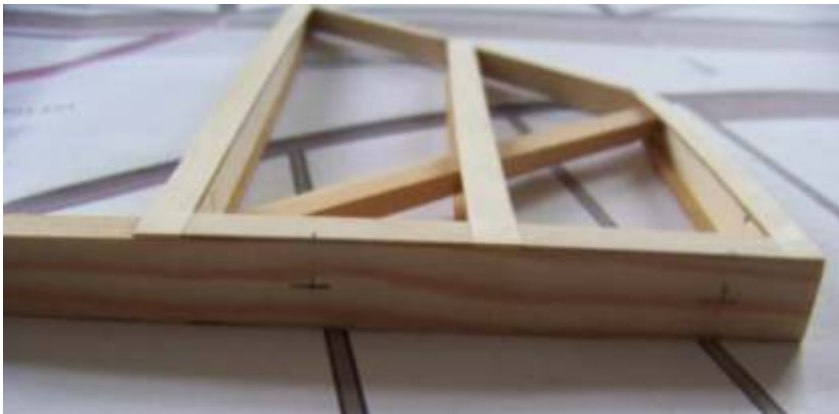
(8) Bore and install the needle hinges. The vertical fin is finished.
