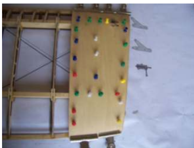
(13) Glue 1mm plywood board (up and down).
