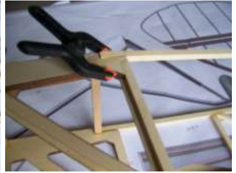
(9) Joint the retral frame of fuselage with battens according to the installation drawing. Then connect it on the fuselage.
