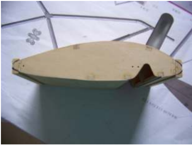
(2) Glue the wood bricks on the front (wider) and back (narrow), and then trim them to be cambered.
