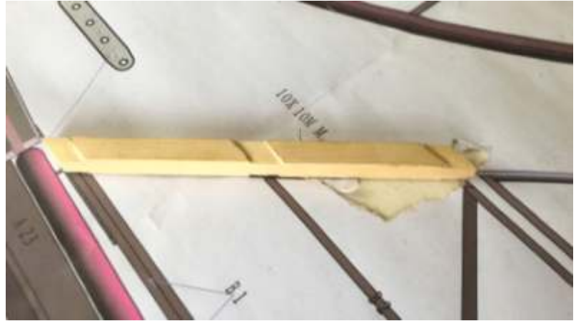
(6) Cut 6 1mm deep grooves (both ends and middle, up and down side) on the vertical fin front batten like the picture, in order to glue 1mm plywood sheet in the grooves.
