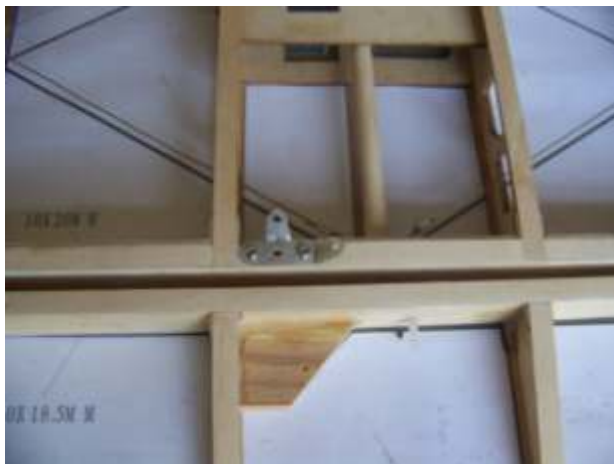
(16) Install the appropriate wood block on the mount of wing strut, and smooth it, then install the metal parts like the pictures.
