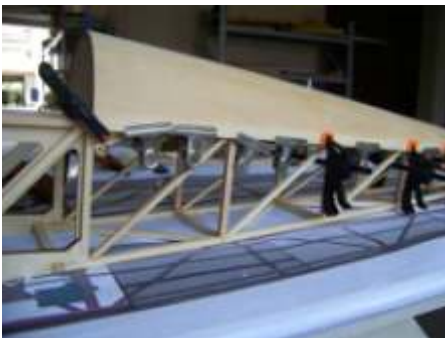
(12) Glue the cover board and fix it with wood sheet to make it more flat.
