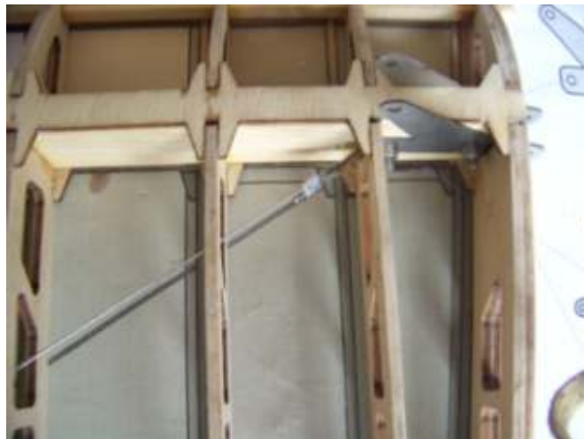
(11) Joint rib E1. And fix the wing on the installation drawing again, then pull \phi 0.8\text{mm} steel wires.
