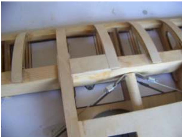
(16) Install the appropriate wood block on the mount of wing strut, and smooth it, then install the metal parts like the pictures.
