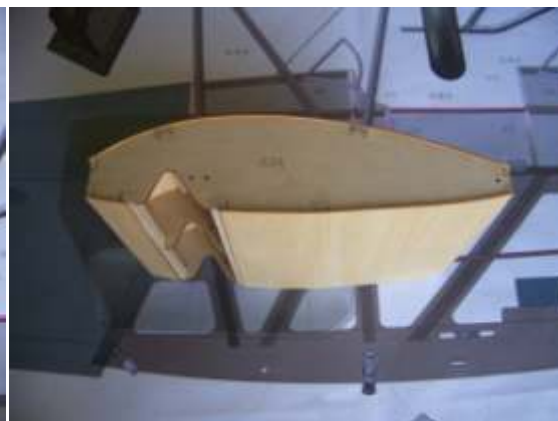
(6) Joint and glue the parts like the picture and then glue the 1mm plywood sheets cover.
