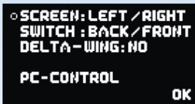
**SCREEN** refers to the position of the OLED screen in the model; **SWITCH** refers to the **SensorSwitch** socket.
